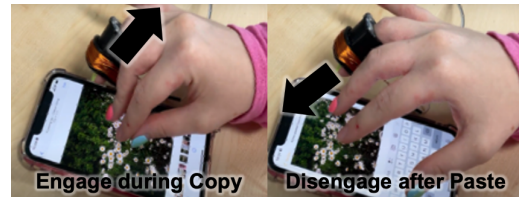
Figure 4: Our ring depicts the status of the interaction by altering the position of the moving guide.
