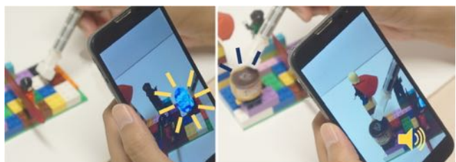
Figure 12. TMotion interacts with the spatially embedded digital contents around the real objects such as discovering hidden virtual character (Left) and playing sounds for different characters (Right).
