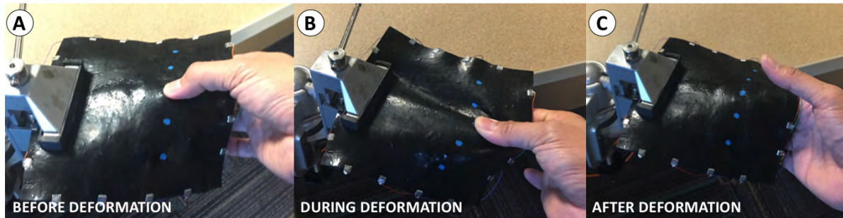
Fig. 11. The step-by-step process for testing localization accuracy upon deformation. (A) Users grasp painted target locations. (B) Users stretch the prototype while grasping the same target location for at least 2 s and (C) release the prototype.
