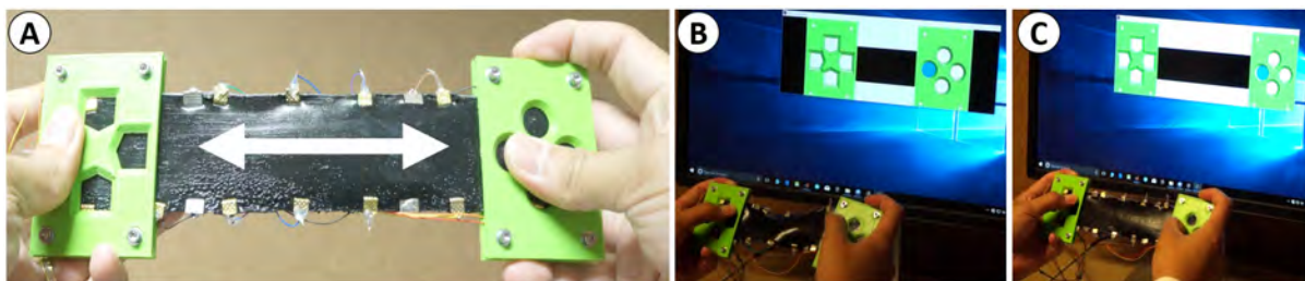
Fig. 15. Contact localization and stretching are embedded for utilizing natural human motions as input metaphors.
